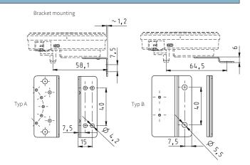
Direct mounting onto armature (fittings)
