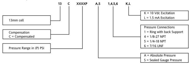
For example: **Part #13C3000PS4K** = 13 mm Cell, Compensated, 3000 psi, Sealed Gauge, 1/8NPT Port with 10 Vdc excitation.
