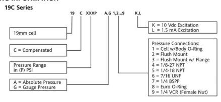
For example: Part #19C100PA4K = 19 mm Cell, Compensated, 100 psi, Absolute, 1/8NPT Port with 10 Vdc excitation.
