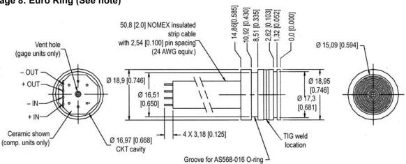
Note: Non-concentricity effects at the diaphragm weld area may cause runout of up to ±0.006 in between the upper and lower portions of the sensor body. (It is recommended to use a counter bore to mate with this device to allow for this nonconcentricity).
