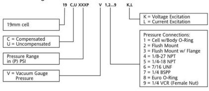
For example: Part #19C100PV4K = 19 mm Cell, Comp., 100 psi, Vacuum Gauge, 1/8NPT Port with 10 Vdc excitation.
