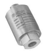
The High Pressure Transducer Model HP is designed to accept extreme pressure ranges of up to 100,000 psi. Equipped with a special blow out plug in its outer case, this transducer will allow the excess pressure to gradually leak out should the pressure element rupture. These transducers operate in a wide temperature range from -65° F through 250° F. Temperature effects on span and zero are 0.005% each and a full scale accuracy of 0.5% is achieved.
