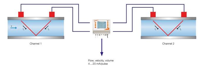
Simultaneous measurement with two pairs of ultrasonic transducers at one common metering point (Compensation of cross-flow effect on measurement, redundancy operation and higher accuracy)
