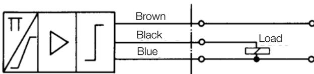
**Connection diagram transmitter TUR-2...M...**
