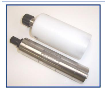
Digiguartz<sup>®</sup> Transducers are incorporated into submersible housings as depth sensors. All depth sensor ranges are available with either frequency outputs or integral intelligent electronics with bi-directional digital communications. Typical application accuracy is better than 0.01% with parts-per-billion resolution, low power consumption, and excellent long-term stability.
