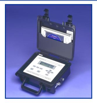
The Model 765 Transfer Standards provide the highest accuracy pressure measurements for portable field applications. The integral Digiquartz<sup>®</sup> Transducers cover absolute pressure ranges up to 40,000 psi (276 MPa) and gauge pressure ranges up to 200 psig (1.38 MPa).
