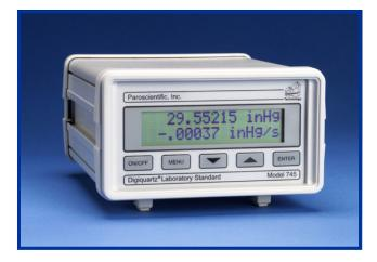
The Model 745 Portable Transfer Standards provide the highest accuracy pressure measurements for laboratory and metrological applications. Digiquartz® Transducers cover 26 absolute and gauge pressure ranges up to 40,000 psi (276 MPa) with unsurpassed accuracy, reliability and stability. The simple, intuitive front-panel user interface and versatile functionality with the rearpanel RS-232 computer interface make the Model 745 the best choice for high performance pressure calibrations.
