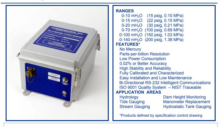
Digiquartz<sup>®</sup> PS-2 Water Stage Sensors provide high accuracy, non-contact water level measurements when used in conjunction with gas-purge bubbler systems. Resolution is parts-per-billion with high accuracy even under difficult environmental conditions. Other desirable characteristics include low power consumption, high reliability, easy installation and low maintenance costs.
