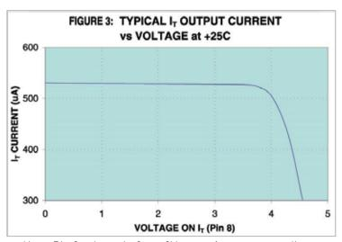
Keep Pin 8 voltage in 0 to +3V range for proper readings.
