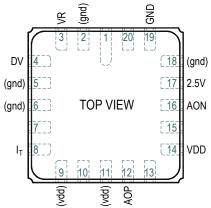
DV (input): Pin 4. Deflection Voltage. Connect to the 2.5 Volt pin for best  $\S$   $\S$   $\S$   $\S$  repeatability. A test input that applies an electrostatic force to the sense element, simulating a positive acceleration. The nominal voltage at this pin is ½ Vop. DV voltages higher than required to bring the output to positive full scale may cause device damage to 2q, 5q, and 10q devices. See app note.
