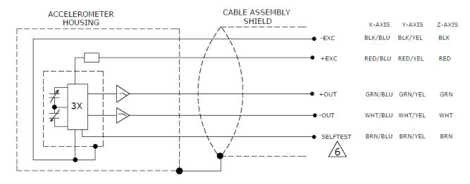
BIT: CONNECT TO CIRCUIT GROUND TO PERFORM SELFTEST WHICH PRODUCES A 24Hz, 1g PEAK-TO-PEAK AMPLITUDE, SQUARE WAVE OUTPUT SIGNAL BY MECHANICALLY ACTUATING SENSOR ELEMENT. THE SELF-TEST OUTPUT SIGNAL IS IN ADDITION TO ANY INERTIAL ACCELERATION ACTING ON THE DEVICE DURING SELF-TEST. A ZERO-G ORIENTATION PROVIDES A ±0.5g SELF-TEST OUTPUT SWING AROUND ZERO-G BIAS. AN AC VOLTMETER DISPLAYS A 0.5g-rms EQUIVALENT OUTPUT SHIFT. A SINGLE-ENDED HOOKUP REDUCES THE SELF-TEST OUTPUT BY HALF.
