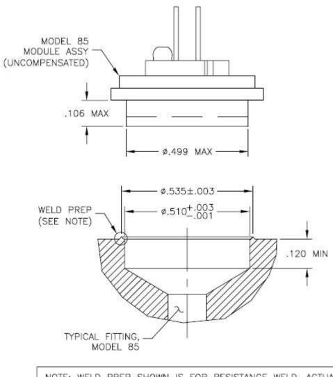
NOTE: WELD PREP SHOWN IS FOR RESISTANCE WELD. ACTUAL GEOMETERY VARIES PER CUSTOMER REQUIREMENTS.
