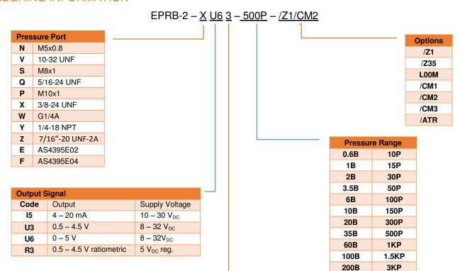
The **psi** range models are only supplied with imperial thread design. The **bar** range models are only supplied with metric thread design.
