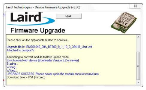
Remove the USB Dongle and re-insert, repeat above steps 3 & 4.
