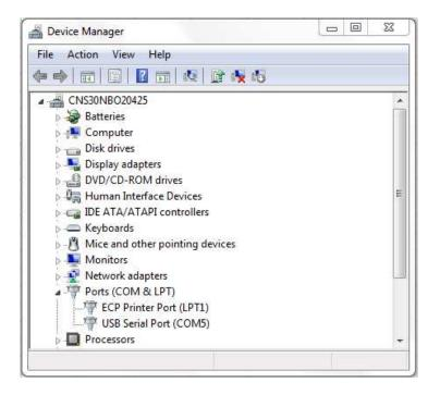
If not assigned, then it is necessary to install the FTDI FT232 USB Serial Converter Driver following instructions from the below link: <u>https://learn.sparkfun.com/tutorials/how-to-install-ftdi-drivers/windows---in-depth</u>
