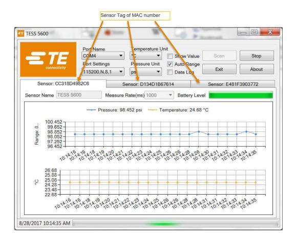
4. Data rate and sensor name can be changed in single unit model (only one sensor selected in scan window). By clicking icon "measure rate", data rate can be adjusted (Default value is 5000ms). And sensor name can be changed by inputing in rectangle.
